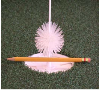
Fig. 1 –StarBall fingers should just touch the top of a pencil for best accuracy.
